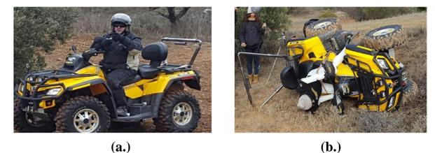
Figure 4. (a.) Air-Quad inoperative position, (b.) Air-Quad active position
