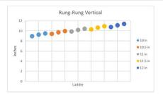
The vertical distance between rungs is dependent on both the rung spacing and the ladder angle. This chart shows these distances for each ladder at each angle. There is a general progression upwards, with a slight dip in distance between the one ladder at its steepest angle to the next larger-spaced ladder at its shallowest angle.
