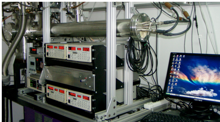
This is a picture of our instrument, called Rapid Single-ultrafine-particle Mass Spectrometer (RSMS), housed inside of our mobile trailer. It is the ability of RSMS to measure the size and composition of particles one-by-one in real-time that facilitates the air quality accountability research that we do.
